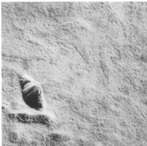
Figure 10 The cone-free surface appearing after 2 h treatment in (50% O 2 + 50% Ar) glow discharge, ×1000.
